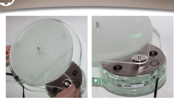
Remove the drive belt and gently place it around the platter and then onto the pulley. It is important to check that your mains supply frequency corresponds to the frequency specified on the Radius 7 mains input label.
