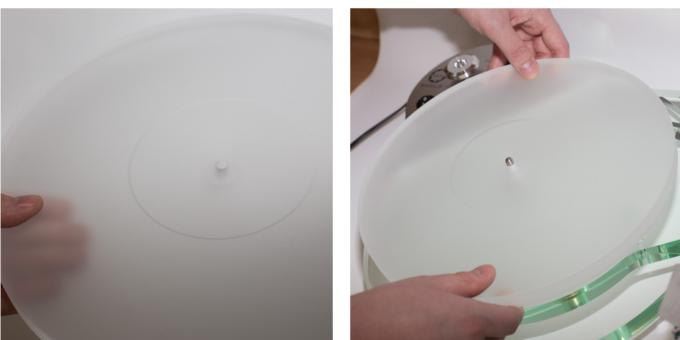
Remove the platter, with the record label recess upper most, carefully locate its central hole over the main bearing spindle and gently lower it until the two are fitted together.
